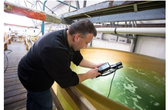
Eudeline monitoring oxygen concentration in growing tanks at the hatchery to investigating water treatment methods.
