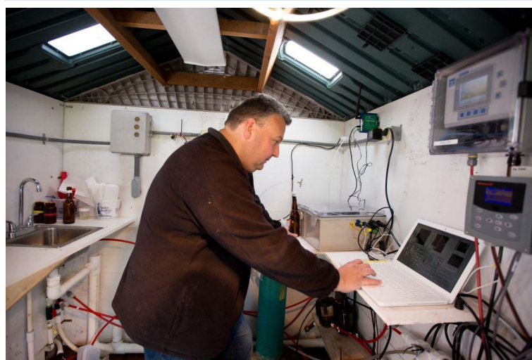
Benoit Eudeline of Taylor Shellfish Hatchery using real-time monitoring equipment that measures pH and water chemistry of seawater.
